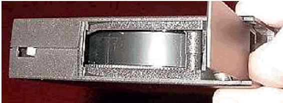
Figure 7: Cartridge leader no longer visible
